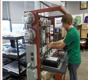
Since the class began this year, I have spent time preparing the training system for classroom use. I connected wires from the solar panel and wind turbine to batteries which store the energy. Wires are then sent through a number of pieces of equipment until it could be converted into energy that can be harnessed and used. Dozens
